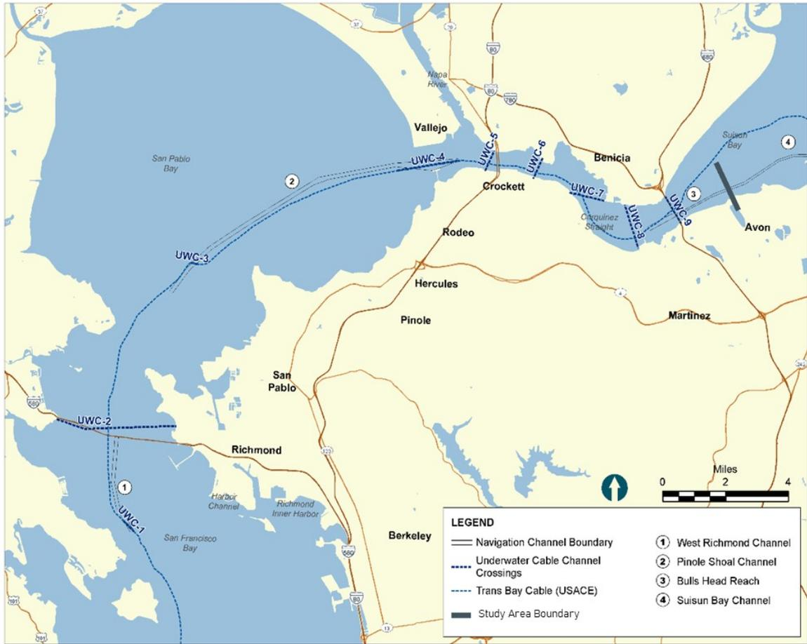
**Figure 2-11. Buried/Underwater Cables.**
